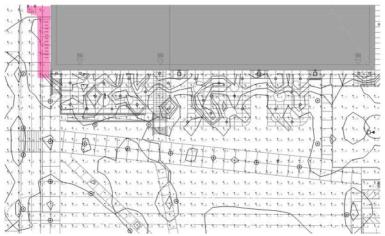
To illuminate the areas highlighted in pink, additional wall packs will be required. We recommend that these additional wall packs be on occupancy sensors to minimize façade illumination. These will be indicated on the plans, complementary to item (a) above.
