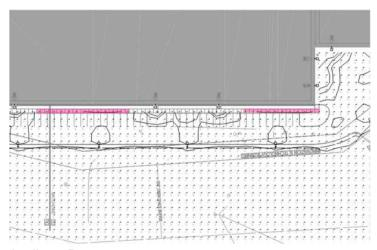
We recommend that these additional wall packs be on occupancy sensors to minimize façade illumination. These will be indicated on the plans, complementary to item (a) above.
